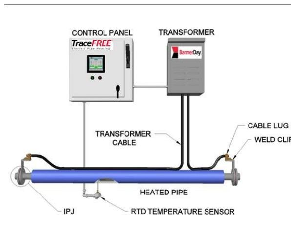
**Electric Pipe Heating System**
